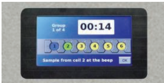
System reminds analyst of sampling time points with visual and audible alerts.
