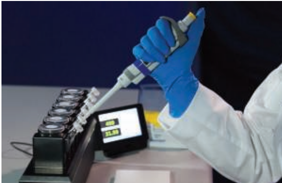
Diffusion testing at Analytic Research Center with Phoenix™ DB-6 manual sampling system.
